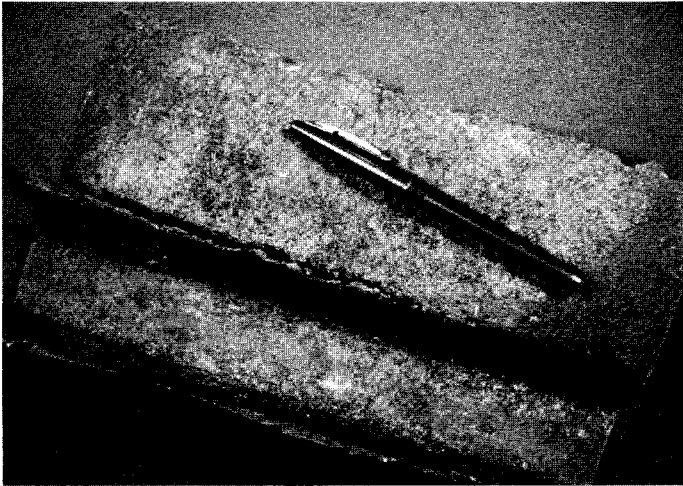
Figure 1 Corrosion-induced separation of top flange from the shoulder (flange/web intersection). Phenolic sample "EP-2" (Table 1) came from this job.
