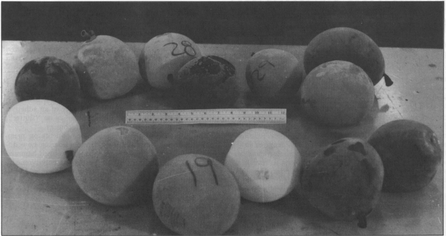
Figure 5 View of some of the balloons used in the test for unrestrained volumetric expansion upon freezing. Note that the 6
