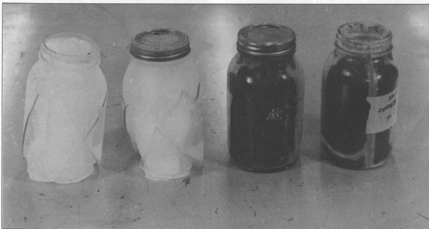
Figure 4 View of 4 of the 10 mason jars used in the test for restrained volumetric expansion upon freezing. Note that two of these jars contain a frozen Sakrete concrete mix and two jars con-
