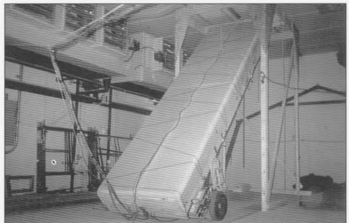
Figure 6. Test roof raised to 44 degree slope in the coldroom.
