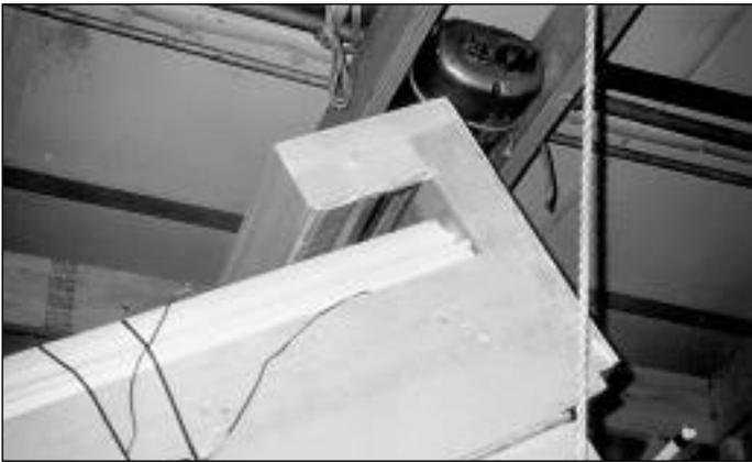
**Figure 17.** Exhaust structure mounted on airways being tested at a slope of 44 degrees.
