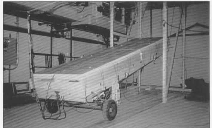
Figure 5. Test Roof raised to 15 degree slope in the coldroom.
