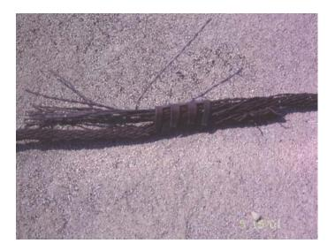
*Figure 9. Frayed conductor strands at a conductor splice. In this condition, the roof membrane is vulnerable to puncture.*
