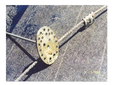
*Figure 14.* View of the underside of a dislodged air terminal. The failure plane was between the base plate and adhesive (i.e., an adhesive failure). See Figure 15.
