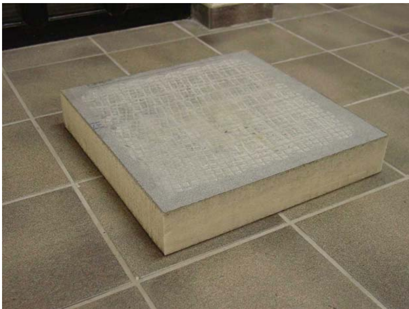
Photo 5. Polyurethane board test specimen after 30 cycles
