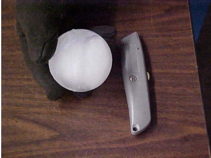
Photo 2: Sphere of frozen ice for impact testing
