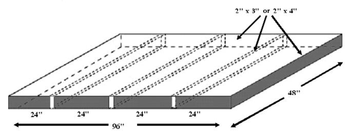
Construct a basic flat deck using 2 x 3 or 2 x 4 dimensional lumber secured with 16-penny nails as shown above. Install one layer ½-inch minimum CDX plywood to deck over the 2 x 4 frame, secured 8 inches on center with 1¼-inch general purpose screws. Install two layers of ¼-inch fiberglass mat-faced gypsum core panel secured with ¾-inch tin capped nails over the plywood. You will need to construct three basic flat deck mockups to conduct the hands-on training exercise.
