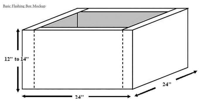
Construct a basic flashing box mockup using four pieces of 2- by 12-inch or 2- by 14-inch dimensional lumber nailed together using 16-penny nails. Add new cant strips for each training session.
