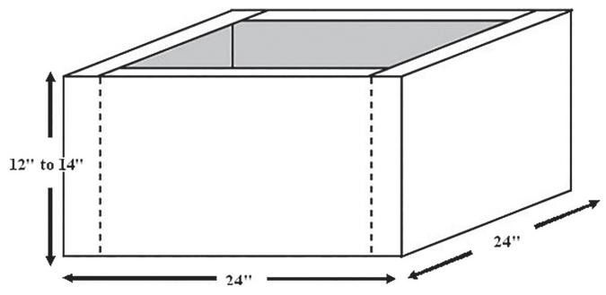
Construct basic flashing box mock-up using four pieces of 2- by 12- or 14-inch dimensional lumber nailed together using 16d nails. Add new cant strips for each training session.
