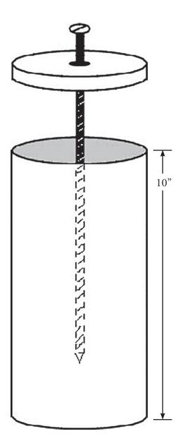
Construct basic pipe penetration mock-up using a minimum 10-inch length of 3- or 4-inch pipe; a circular plywood disk cut to size of the outer pipe diameter; and a screw 2 inches longer than the pipe length. Drill a hole near the center of the plywood disk to accept the screw. Secure the basic pipe penetration mock-up at the opposite end of the basic deck mock-up approximately 18 inches from one side and 24 inches from the end. The basic pipe mock-up can easily be removed for storage.
