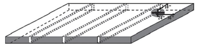
Cut a hole 18 inches from one side and 18 to 24 inches from one end in two of the three basic flat deck mock-ups. Use a 9-inch metal pie tin, a large coffee can or an inverted galvanized steel tall cone flashing cut to height to simulate a roof drain opening. Secure the simulated roof drain in the hole.
