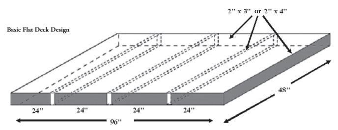
Construct basic flat deck using 2x3 or 2x4 dimensional lumber secured with 16d nails as shown here. Install one layer ½-inch minimum CDX plywood to deck over the 2x4 frame, secured 8 inches on center with 1½-inch general-purpose screws. Install two layers of ¼-inch fiberglass mat-faced gypsum core panel secured with ¾-inch tin-capped nails over the plywood. You will need to construct three basic flat deck mock-ups to conduct the hands-on training exercise.
