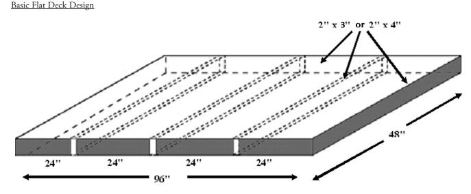
Construct a basic flat deck using 2 x 3 or 2 x 4 dimensional lumber secured with 16-penny nails as shown above. Install one layer ½-inch minimum CDX plywood to deck over the 2 x 4 frame, secured 8 inches on center with 1¼-inch general purpose screws. Install two layers of ¼-inch fiberglass mat-faced gypsum core panel secured with ¾-inch tin capped nails over the plywood. You will need to construct three basic flat deck mockups to conduct the hands-on training exercise.
