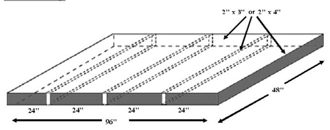
Construct a basic flat deck using 2 x 3 or 2 x 4 dimensional lumber secured with 16-penny nails as shown above. Install one layer ½-inch minimum CDX plywood to deck over the 2 x 4 frame, secured 8 inches on center with 11/4-inch general purpose screws. Install two layers of 1/4-inch fiberglass mat-faced gypsum core panel secured with 3/4-inch tin capped nails over the plywood. You will need to construct three basic flat deck mockups to conduct the hands-on training exercise.
