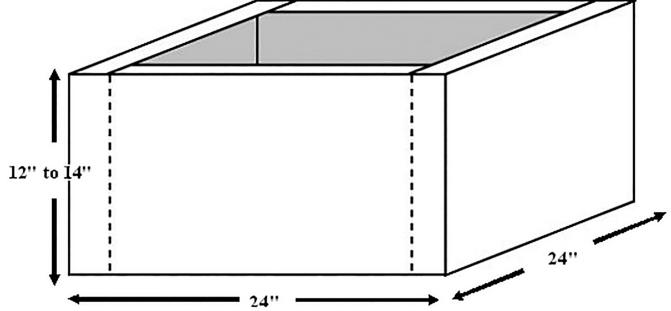
Construct a basic flashing box mockup using four pieces of 2- by 12-inch or 2- by 14-inch dimensional lumber nailed together using 16-penny nails. Add new cant strips for each training session.
