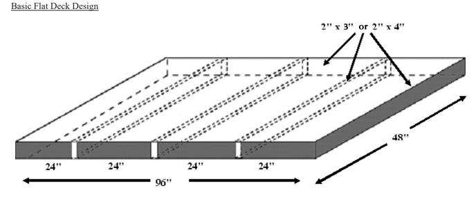
Construct a basic flat deck using 2 x 3 or 2 x 4 dimensional lumber secured with 16-penny nails as shown above. Install one layer  $\frac{1}{2}$ -inch minimum CDX plywood to deck over the 2 x 4 frame, secured 8 inches on center with 11/4-inch general purpose screws. Install two layers of 1/4-inch fiberglass mat-faced gypsum core panel secured with 3/4-inch tin capped nails over the plywood. You will need to construct three basic flat deck mockups to conduct the hands-on training exercise.
