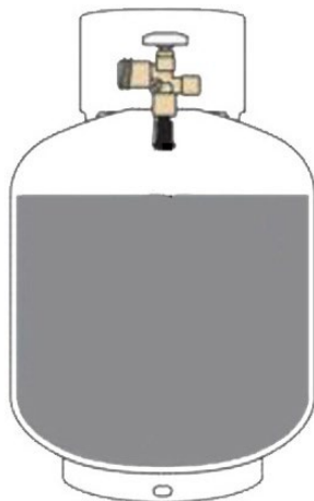
Figure 4: Vapor collects at the top of a tank.
