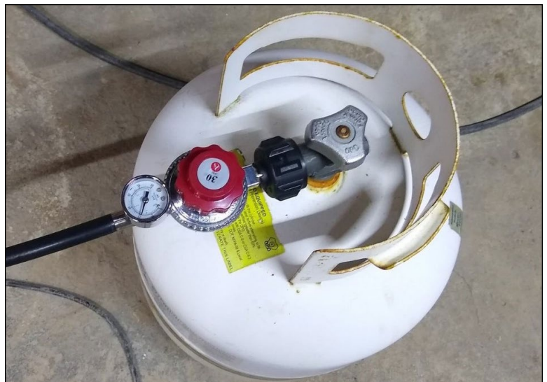
Photo 6: Adjustable pressure regulator assembly
