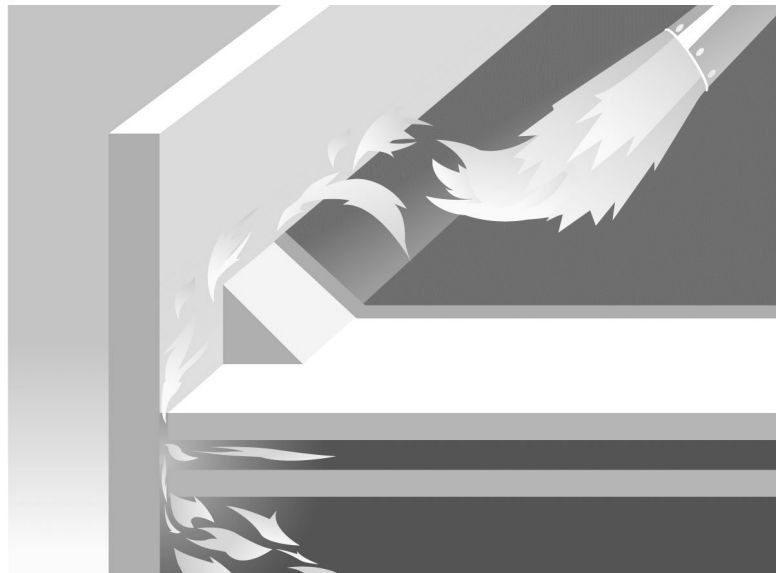
Figure 1: Extend base plies a minimum of 3 inches.
