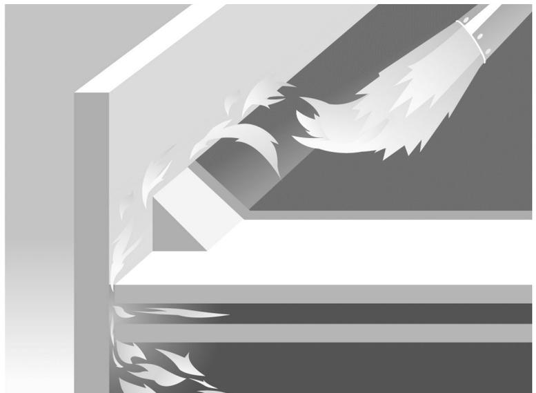
Figure 1: Extend base plies a minimum of 3 inches.
