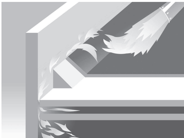
Figure 1: Extend base plies a minimum of 3 inches.
