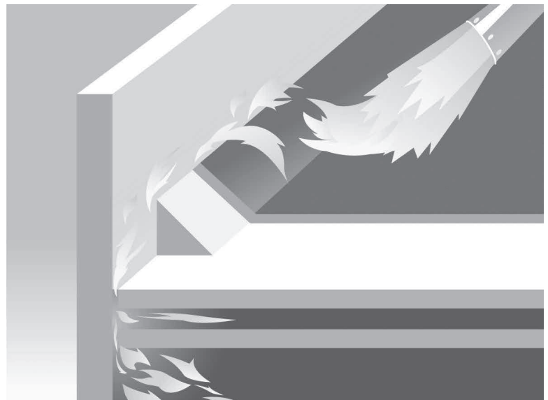
Figure 1: Extend base plies a minimum of 3 inches.
