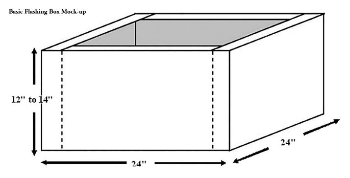
Construct basic flashing box mock-up using four pieces of 2- by 12- or 14-inch dimensional lumber nailed together using 16d nails. Add new cant strips for each training session.
