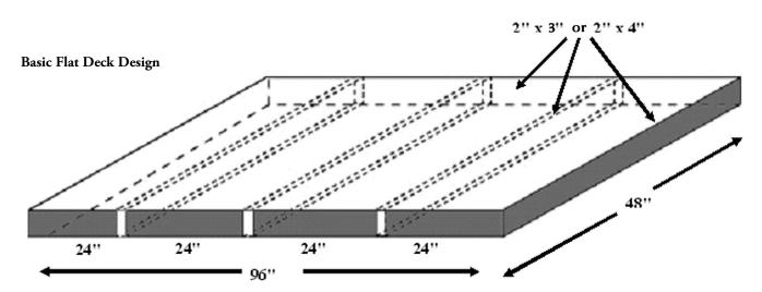
Construct basic flat deck using 2x3 or 2x4 dimensional lumber secured with 16d nails as shown here. Install one layer ½-inch minimum CDX plywood to deck over the frame, secured 8 inches on center with 1½-inch general purpose screws. Install two layers of ¼-inch fiberglass mat-faced gypsum core panel roof insulation secured with ¾-inch tin-capped nails over the plywood. You will need to construct three basic flat deck mock-ups to conduct the hands-on training exercise.
