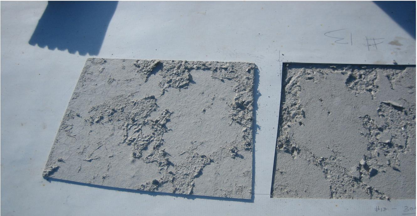
Photo 5 The new construction in a western state had a fully adhered roof system, white membrane and gypsum cover board. Moisture from the lightweight structural concrete deck drove up into roof system, wetting the cover board.
