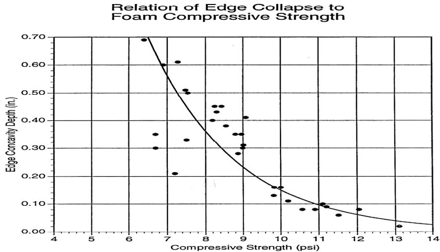
Using this graph and correlating processing parameters and formulations it is possible to manufacture boards with acceptable compressive strengths (called ZCS – Z Direction Compressive Strength) and therefore a board with little or no cuppage / edge collapse.
