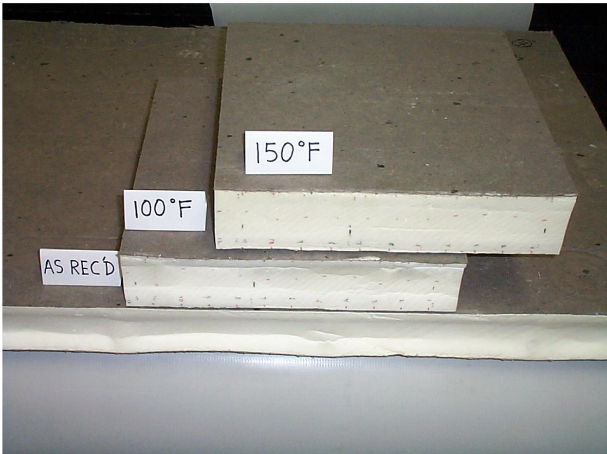
Measurement of the ZCS during production, however, is limited because of the time needed to cut the appropriate sample and measure it. Typically, this means only one or two boards are tested per batch and then not the entire 2.4-meter (8-foot) edge of each board is tested - only a section.
