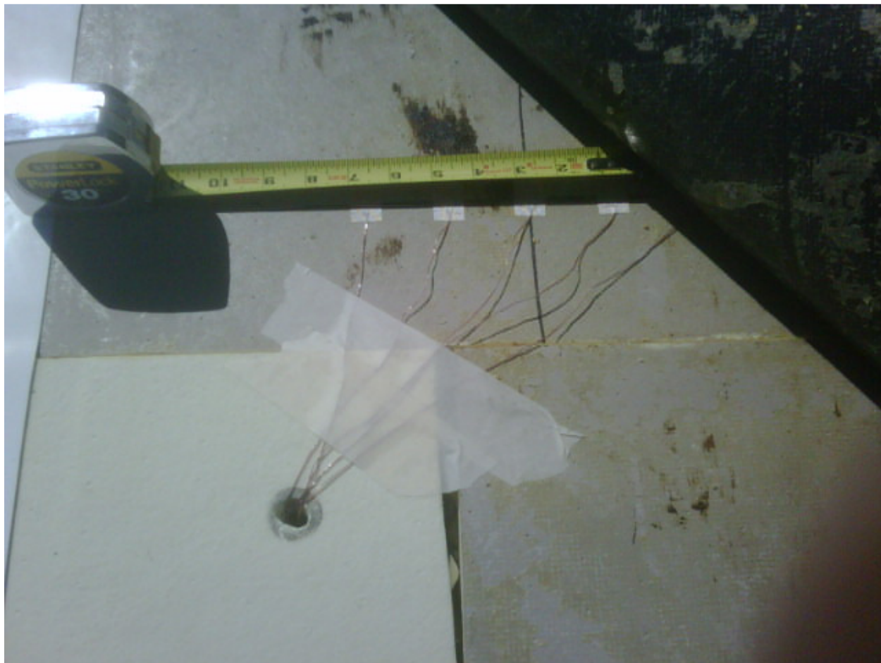
Photo 3. View of the thermocouple array, during installation, which traverses from white TPO to under the PV panel as diagramed in Photo 4.
