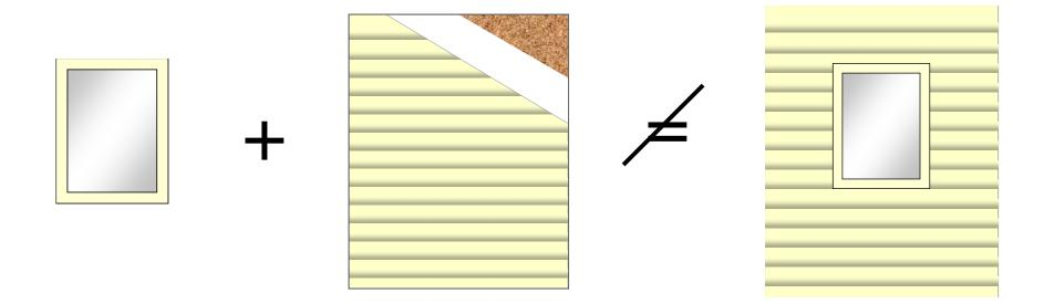
Significant effort has focused on the development of installation methods that are standardized and tested at the window / wall interface as an installed system.
