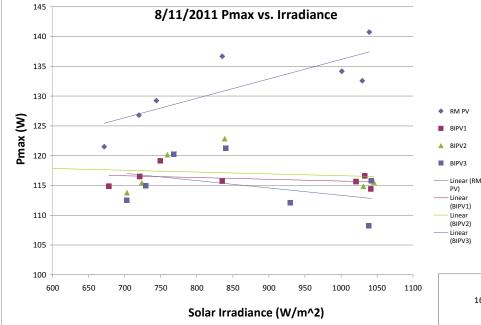
On a cooler day with similar irradiance, see a positive trend with Pmax vs Irradiance for all systems, but still a ~15% reduction in PV output for the BIPV Systems
