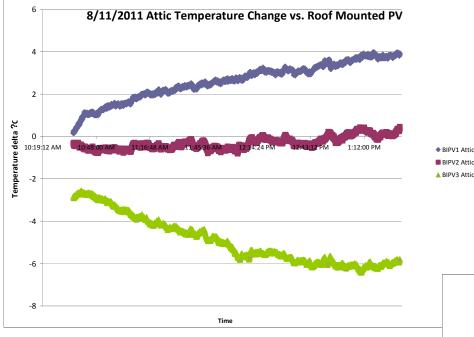
BIPV Attic Temp Difference (compared to Roof Mounted Control): Unconditioned Attic shows moderate temperature rise, whereas Fully Conditioned Attic Temp is cooler than all other systems
